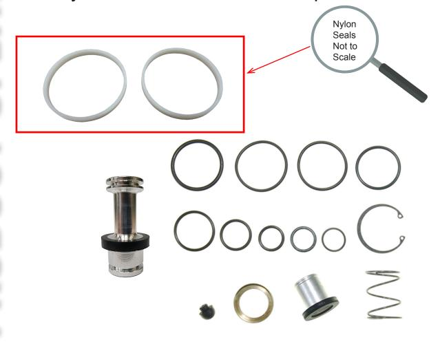
Order kit BEN702997M, major repair kit for HR-1 Type Valve. This kit is used to repair 065060 and 065147 valves.
