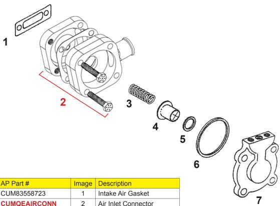
CUM83558723 **CUMQEAIRCONN** CUM83049553 3 **Unloader Spring** CUM8184240 4 **Unloader Cap** 5 CUM8127936 Vee Seal CUM83043995 Unloader O-Ring 6 CUM83558828 7 **Unloader Body**
